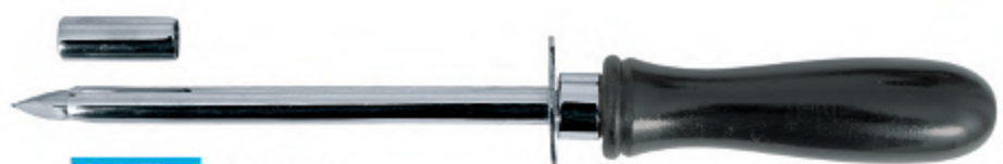
01-1173 Bloat Trocar The flat-to-round shape has made this wooden-handled trocar very popular for venting animal gas accumulations. Includes stainless steel cannula and protector cap. Cannula length is 6". Also available in 5" length.
