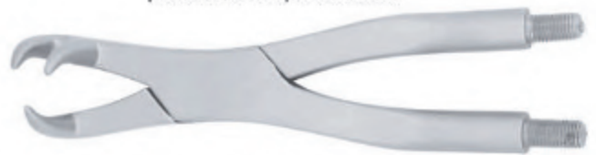
01-1078 3 Root Box Joint Forceps Off Side With knurled handles. For molars with very little crown in aged horses and deciduous premolar caps. Length 19" s/s.
